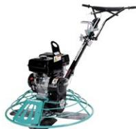
The J36K65 / SXH 4 Blade Power Trowel, with a 36" diameter (90cm), M. Kohler 6.5 HP, 60 to 125 RPM, weight 68 Kgs. Standard handlebar. Its front access panel provides quick reach to the trowel arms and blades. Its spider and push collar mounting design simplifies routine maintenance. The gearbox features premium components and large oil capacity for years of trouble-free operation.
